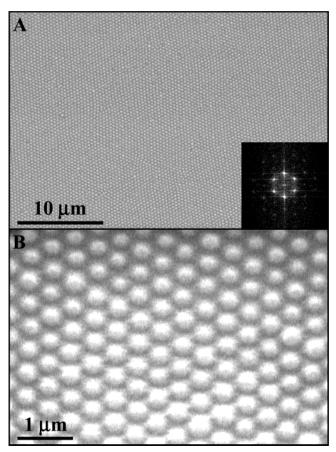
**Figure 2.** Typical scanning electron microscope (SEM) images of a spincoated colloidal crystal-polymer nanocomposite film. (A) Top-view image of the sample in Figure 1. The inset showing a Fourier transform of a 40  $\times$  40  $\mu$ m region. (B) Higher magnification SEM image of the same sample.
