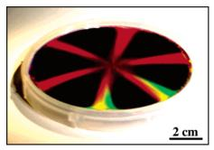
**Figure 1.** Photograph of a 3D ordered nanocomposite film on a 4-inch silicon wafer illuminated with white light. The sample is made from 325 nm diameter colloidal spheres and spin-coated at 600 rpm for 120 s.
