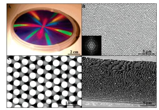
*Figure 7.* Formation of wafer-scale colloidal crystals by selective removal of polymer matrix. (A) Photo of a released colloidal crystal on a 4-inch silicon wafer. (B) Typical SEM image and its Fourier transform (inset) of the above sample. (C) Higher magnification image. (D) Cross-sectional SEM image.
