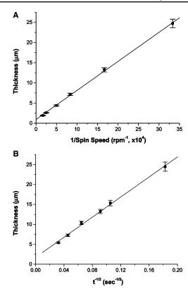
**Figure 6.** Precise control of the crystal thickness. (A) Linear relationship of the crystal thickness vs the inverse of the spin speed at constant coating time, 120 s. (B) Film thickness vs the inverse of the square root of spin time at constant spin speed, 600 rpm. 325 nm diameter colloids are used for all cases.
