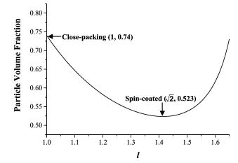
**Figure 10.** Relationship between particle volume fraction of possible crystals during vertical compressing vs the ratio, *l*, of in-plane particle center-to-center distance to the sphere diameter.
