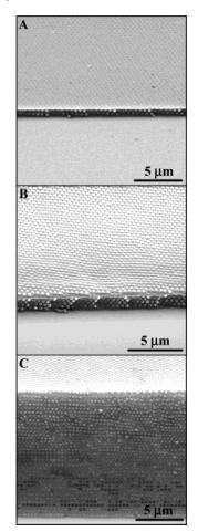
*Figure 4.* Typical side-view SEM images of spin-coated nanocomposite films with different thickness. (A) A 2-layer sample coated at 6000-rm for 900 s. (B) A 5-layer sample coated at 6000-rpm for 170 s. (C) A 41-layer sample coated at 600-rpm for 120 s 325 nm diameter colloids are used for all cases.
