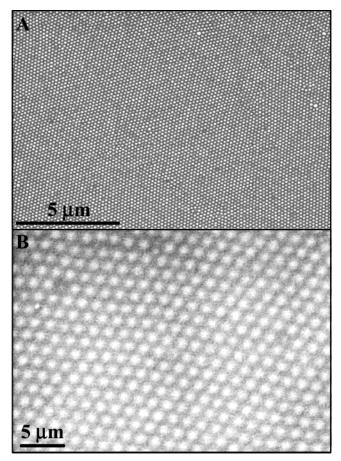
*Figure 5.* Typical top-view SEM images of spin-coated nanocomposite films with different sphere sizes. (A) A sample made from 130 nm diameter spheres and coated at 600 rpm for 120 s. (B) A sample made from 1320 nm diameter spheres and coated at 600 rpm for 120 s.
